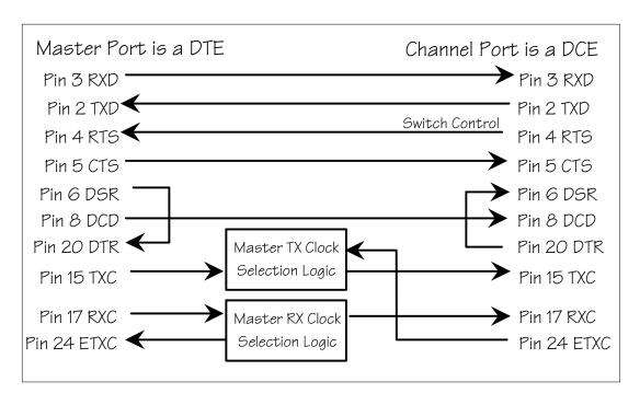
Master DTE / Sub-Channel DCE Interface Flow Diagram
